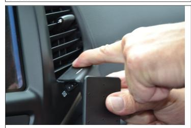
3. The seam between the vent frame and inside of the vent is a tight seam. To make the upper angled edge of the ProClip go all the way into the seem between the air vent and the surrounding panel frame, pull the ProClip towards you and press down at the same time. It might need to be wiggled a little. Listen for the click as the ProClip goes into place.
