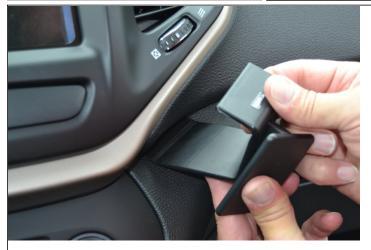
1. Peel off the cover of adhesive tape on the ProClip. Place the ProClip over the area where it will be attached for proper alignment. The ProClip label (sticker) is on the top. Place your finger at the bottom edge to mark the placement.
