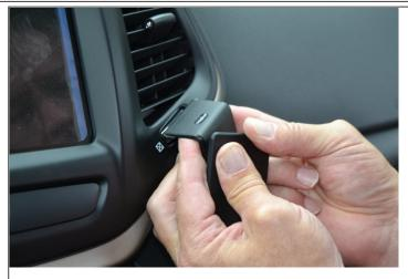
2. Rotate the ProClip upward so the angled edge on the lower part hooks behind the lower dashboard panel. Then place your index fingers underneath the upper part of the ProClip and pull upward to hook the upper angled edge of the ProClip over the air vent edge.
